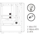
Please make sure that the motherboard aims at the copper cylinder and fix motherboard with No.3 screw.
