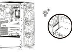
Remove the baffle marked in the picture, make sure the VGA card aims at the motherboard slot and then fix VGA card and case with No.1 screw.
